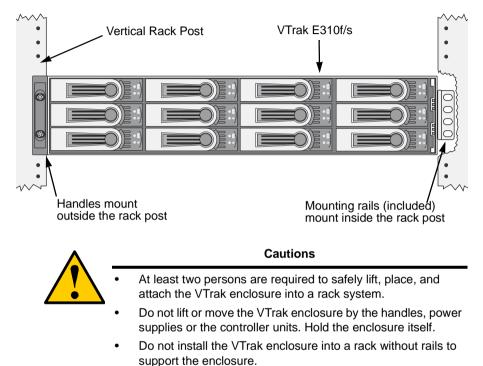
To install the VTrak enclosure into a rack with the supplied mounting rails:
